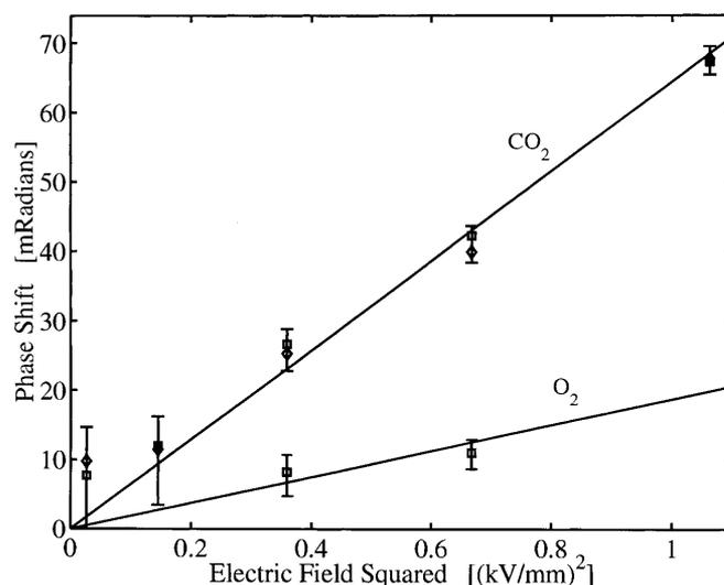
**Fig. 3.** The Kerr-induced phase shift as a function of the square of the electric field. Both gases are at  $P = 1$  atm
