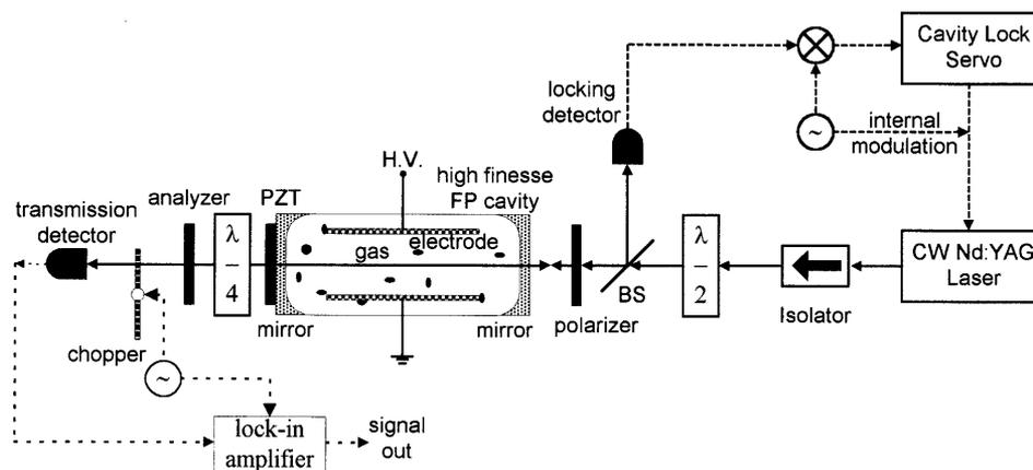
**Fig. 1.** Experimental setup for measurements of the Kerr effect in gases using a Fabry–Pérot-based ellipsometer. BS – beamsplitter, PZT – piezo electric transducer, H.V. – high voltage
