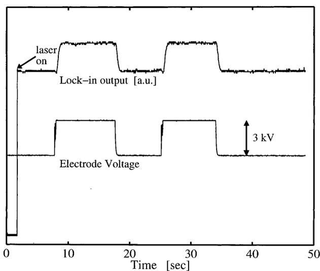
**Fig. 2.** The output signal of the ellipsometer with and without the high voltage, as a function of the time. The measured gas is  $\text{CO}_2$  at a pressure of 1 atmosphere and a voltage of 3 kV applied to the electrodes
